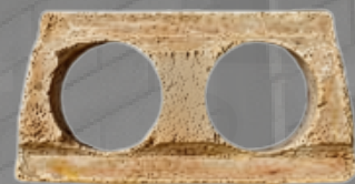
REHIB - REGULAR EXTRA HOLLOW INTERLOCKING BRICK
